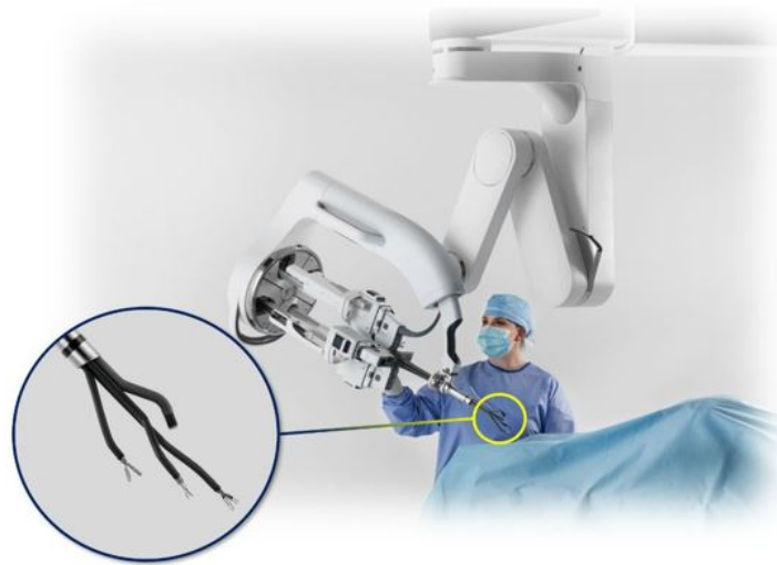
Figure 1: Da Vinci SP consisting of multiple flexible instruments and an endoscope emerging through a single cannula. Image source: Intuitive Surgical, Inc.
