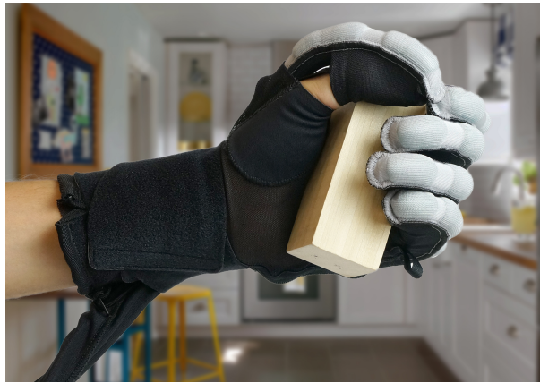
Figure 5: Soft Robotic Glove for Neuromuscular Rehabilitation (credits: Wyss Institute at Harvard University)
